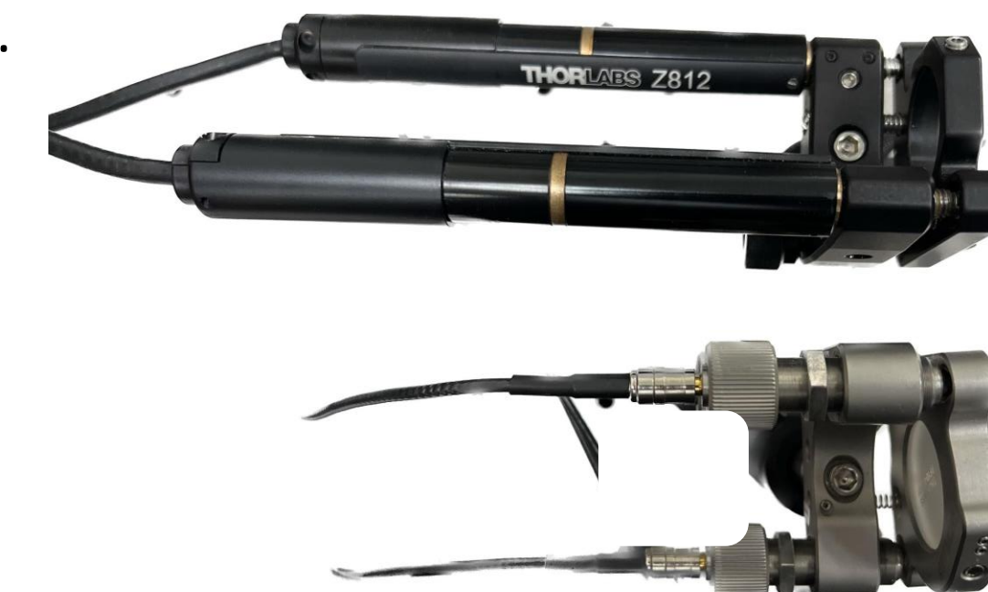
Size comparison of DC Servo Mirrors Thorlabs Kinematic Mounts - KS1T (top) and Piezoelectric Mirrors Thorlabs Polaris Mounts - K1S3P (bottom).
